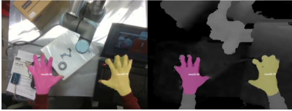
Fig. 6.13 Typical results obtained from an opaque industrial scene with RGB-D input (RealSense D435i) and SOLOv2 ResNet50
