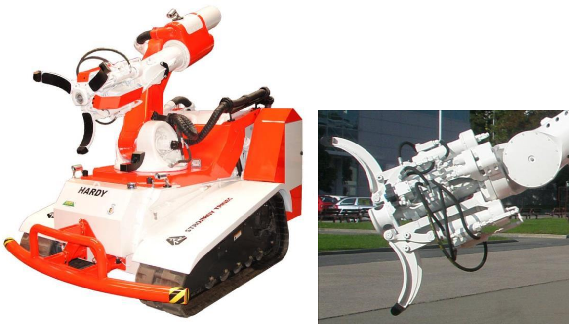
Fig. 6.38: Robot Hardy (left), Robot gripper without shields with the integrated water nozzle (right)
