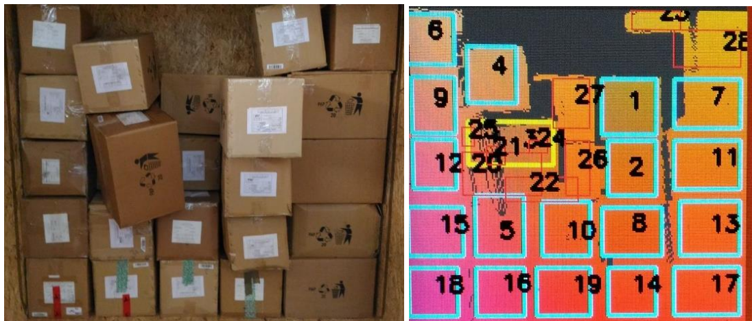
Fig. 6.40: HW and SW system for recognition of boxes in a container. Digits indicate the proposed order of collection.
