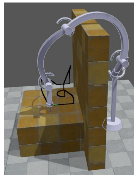
Fig. 6.22: Example of a proposed general optimal kinematic structure with curved arms
