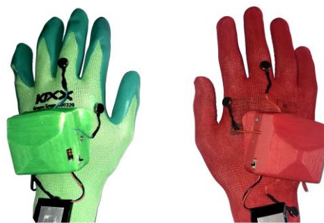
Fig. 6.10: Prototype of the notification devices. Each glove is equipped with six vibration motors, which provide haptic feedback
