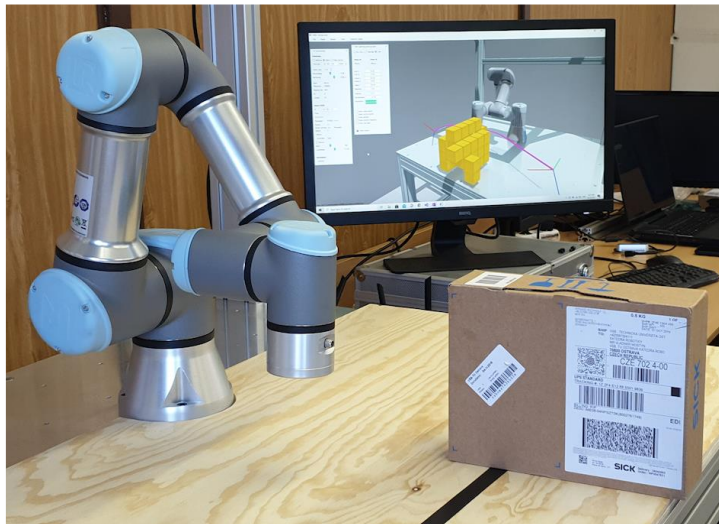
Fig. 6.20: Practical testing of the obstacle avoidance algorithm using an imaginary elastic band, in the foreground the real workplace, in the background the control system with 3D real-time visualization
