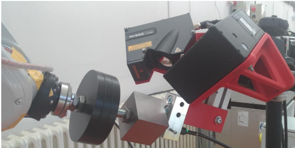
Fig. 6.3: Measuring nest. A robot with the payload tool approaches to confocal sensor that measures the TCP Z-axis distance. TCP X and Y are measured by a pair of laser profilers above the payload tool.
