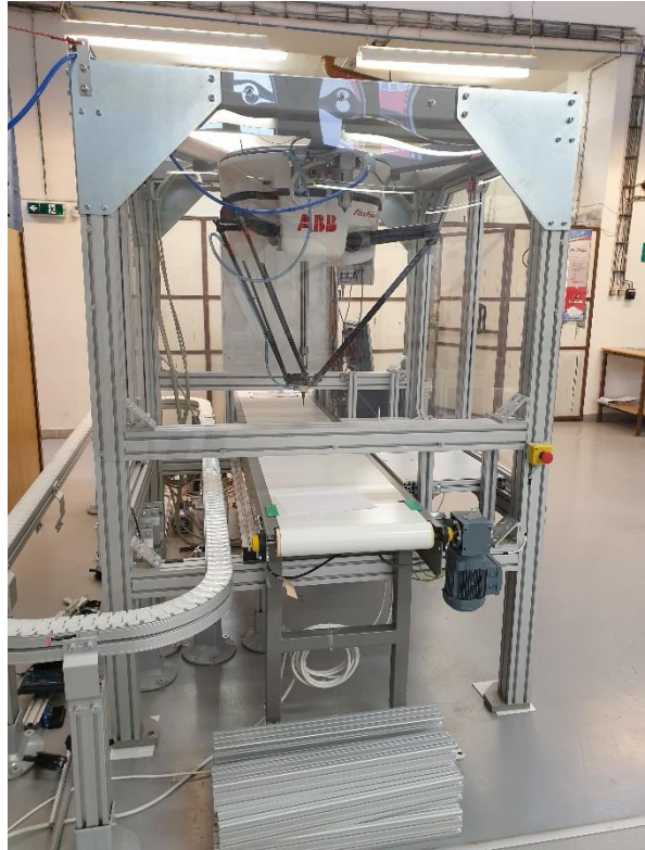
Fig. Robotized workplace with ABB IRB360 robot, conveyors and machine vision system
