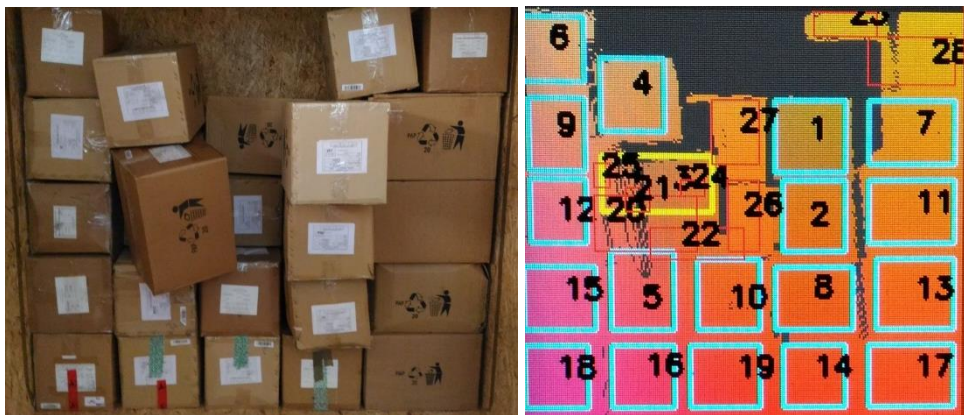
Fig. HW and SW system for recognition of boxes in a container. Digits indicate the proposed order of collection.
