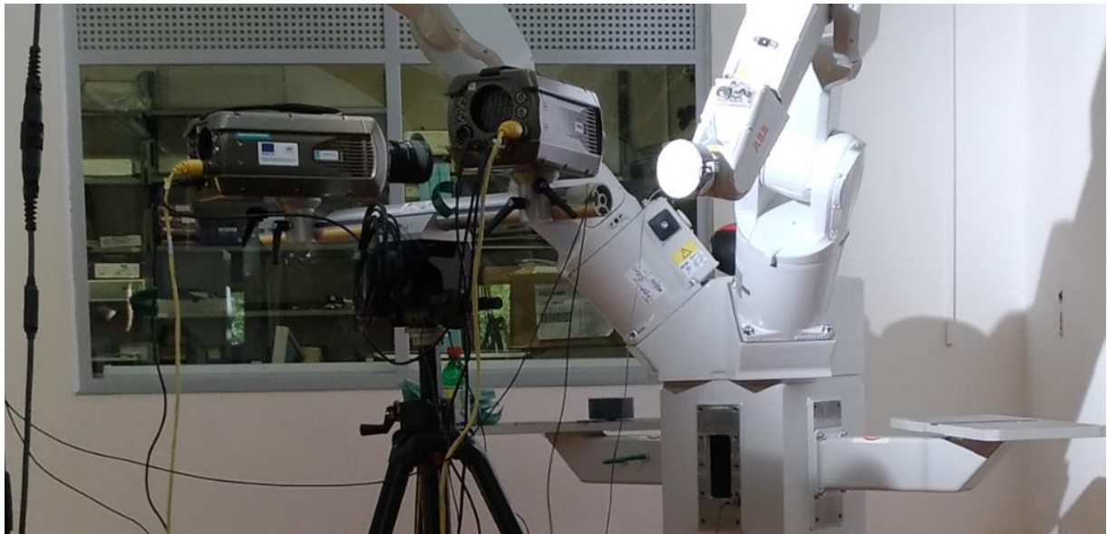
Fig. Use of DANTEC DIC cameras to measure the repeatability of the manipulator
