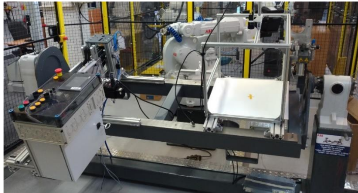
Fig. Upcoming test robotic workplace for assembly of rubber profile on sleeve molding to verify the functionality of the feeder prototype
