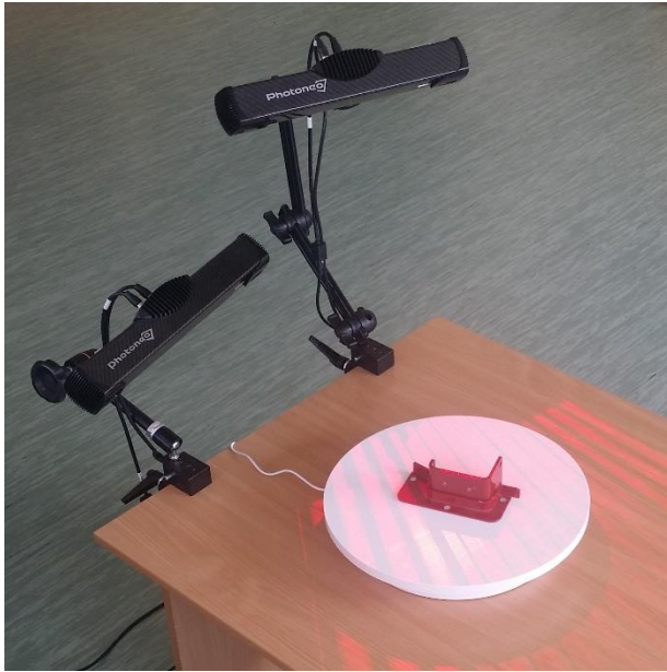
Fig. Scanning system when creating a 3D scan
