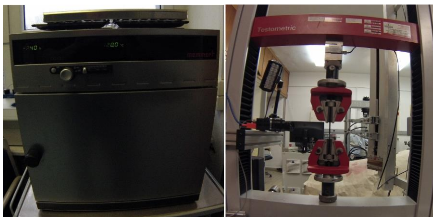
Fig. Industrial oven (left), test machine with tearing test sample (right)
