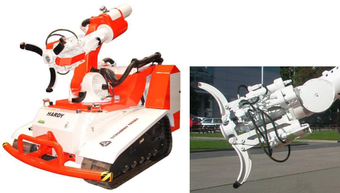
Fig. Robot Hardy (left), Robot gripper without shields with the integrated water nozzle (right)
