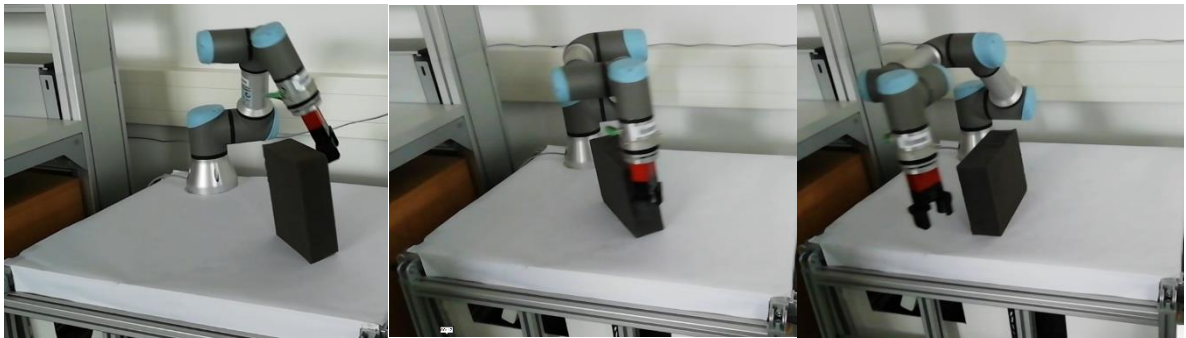
Fig. Collision of the robot with an obstacle
