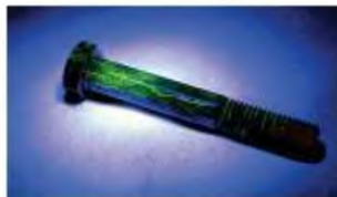
Obr. 5: Trhliny na šroubu nalezené pomocí MT kontroly Zdroj: https://www.qualitymag.com/articles/95878-magnetic-particle-inspection-performance
