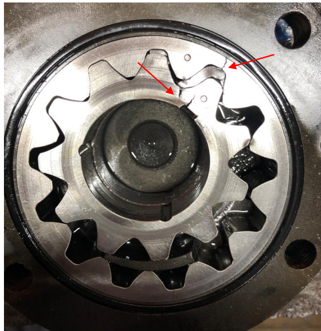
Fig. 4.5 An example of damage due to impurities in a hydraulic system with external gear hydraulic pump
