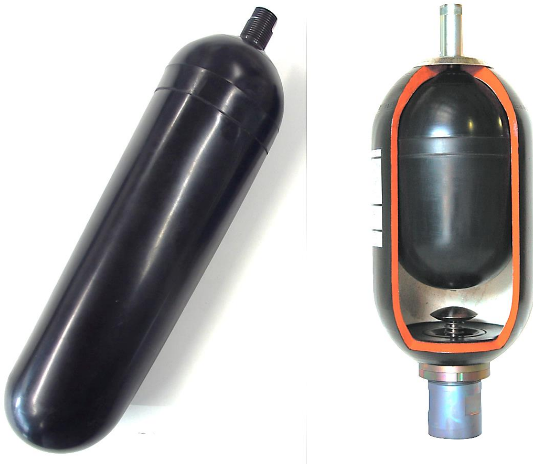
Fig. 10.9 Bladder of accumulator (left), bladder accumulator in cut (right) [63]
