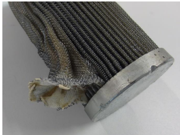
Fig. 4.13 Low-pressure filter with optical-electrical signalization of filter element contamination indicator (left), damage to the filter element when the filter was incorrectly connected to the hydraulic system (right)
