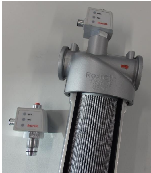
Fig. 4.13 Low-pressure filter with optical-electrical signalization of filter element contamination indicator (left), damage to the filter element when the filter was incorrectly connected to the hydraulic system (right)
