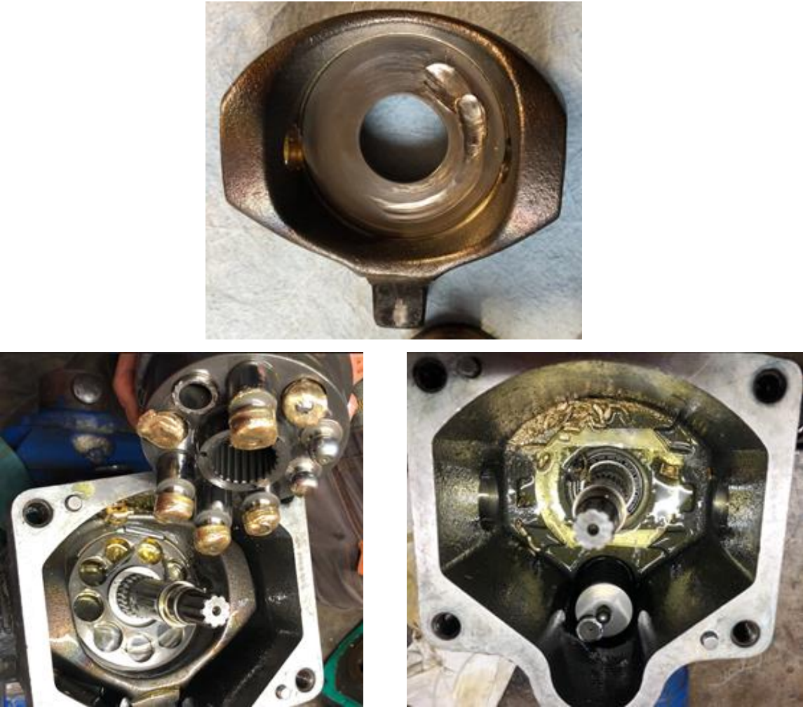
Fig. 2.4 Damage to the axial piston hydraulic pump due to a reduced lubricating liquid ability
