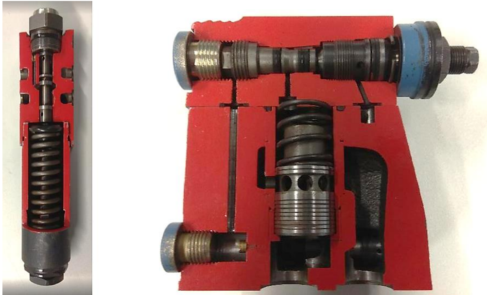
Fig. 9.10 Seat construction direct operated pressure reducing valve (left), seat construction pilot operated pressure reducing valve (right)
